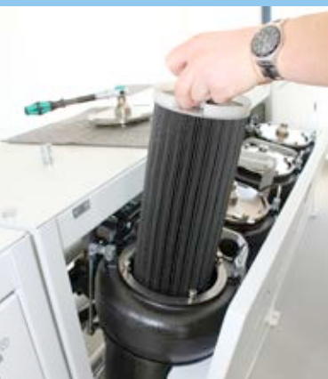
The filter cartridges are regularly backflushed parallel to the process. In case of wear, they can be replaced cleanly and in a very short time.
