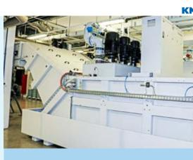
Central cleaning system for aqueous solution: KNOLL combines hydrocyclones and MicroPur® filters (in the foreground at the top) in order to supply a total of 40 indexable insert and separating machines with 3500 l/min cleaned aqueous solution at Ceratizit Austria.
