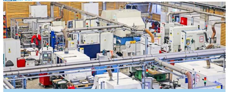
A look into a production hall at Ceratizit Austria, where carbide metal indexable inserts are ground. The superfine cleaning of the grinding oil is indispensable for their high quality.
