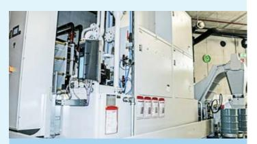
Ceratizit Austria has had excellent experiences with KNOLL Micro-Pur® central systems for oil cleaning. The filter fineness is 1  $\mu$ m, and the gravimetric residual dirt content dropped from 100 mg/l to just 1 mg/l.
