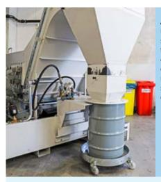
An important component of the KNOLL filter systems is the integrated, automatic sludge concentrator, which ensures that the carbide metal sludge lands squarely in the disposal drum.
