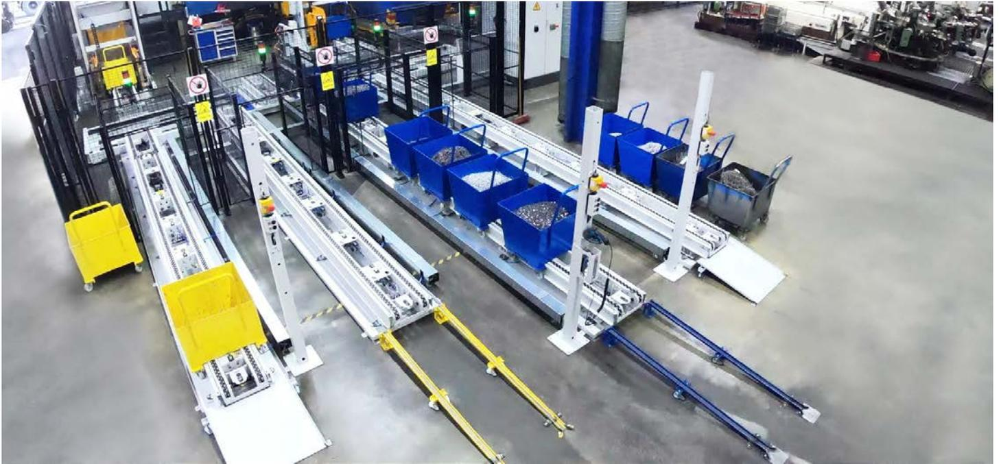
The chip centrifuges are arranged behind the KNOLL transport systems. From there, the degreased chips are taken to the appropriate containers to the right via a portal.
