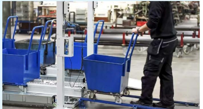
It takes only 10 to 15 seconds to move a swarf trolley into the system and remove another one from it.
