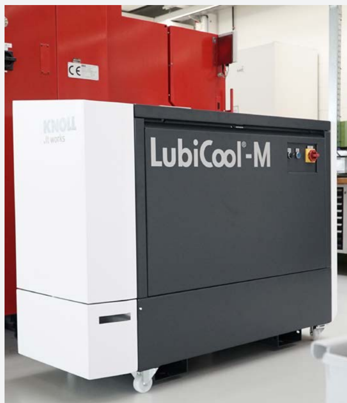
The mobile high-pressure station KNOLL LubiCool®-M generates a cooling lubricant pressure of up to 150 bar and a flow rate up to 27 l/min.
