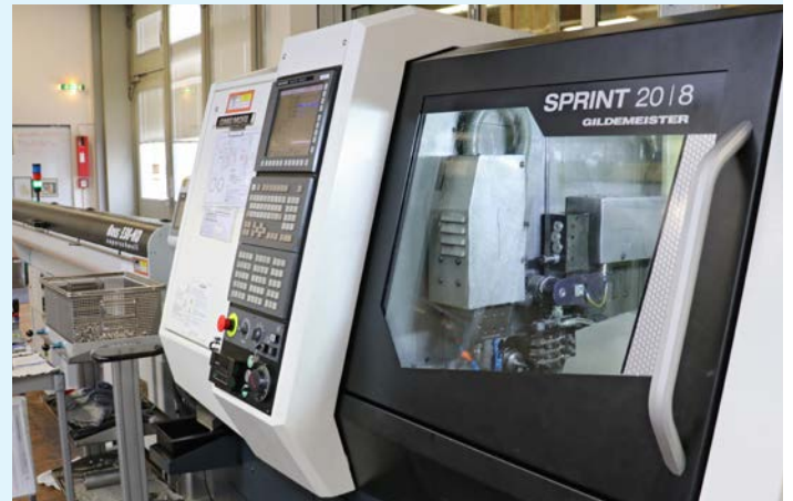
The SPRINT 20 from DMG MORI used as a fixed headstock lathe: With this machine, ifm produces adapter pieces in three-shift operation for fluid sensors.
