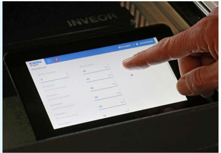
A highlight of the entire LubiCool® range is the incredibly simple and intuitive operation. For this, KNOLL developed the new "SmartConnect" control concept, which includes a small touch display, via which the user can set and adjust the desired pressure level and other parameters.
