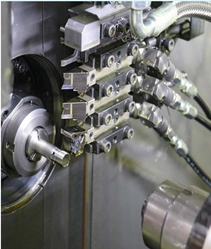
Up to eight switchable outputs on the KNOLL LubiCool®-S high-pressure unit ensure that the machine tool - in this case, the DMG MORI SPRINT 20 - is supplied with cooling lubricant as required.
