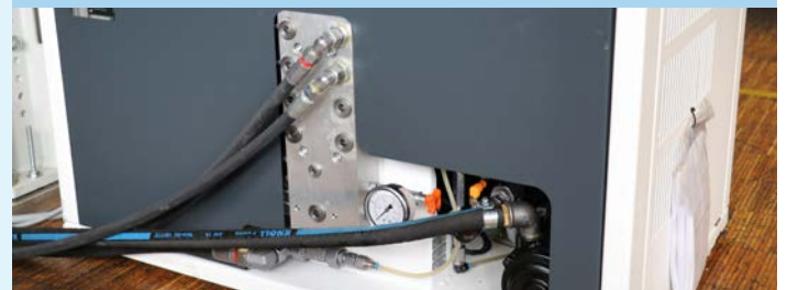
LubiCool®-S from the back: KNOLL supplies the high-pressure system for plug-and-play - complete with hose package, accessories and machine-specific interface.
