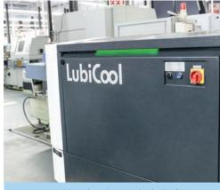
KNOLL Maschinenbau has packed all of its extensive expertise regarding the high-pressure cooling lubricant supply of automatic lathes into the mobile LubiCool® unit.
