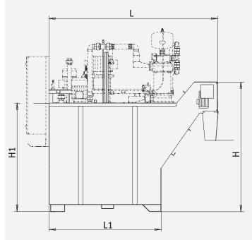
Depicted is a system with lifting pump, TURBO reversible flow filter, filtered fluid tank, supply pumps and control
