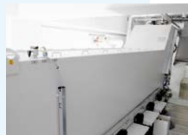
The additional automatic concentrator ensures the recovery of the valuable metal carbide chips from the back-flush product of the MicroPur® filter. With this filter, the KNOLL system achieves a very low oil carry-over.
