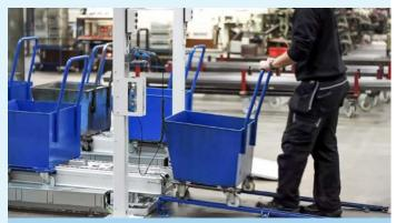
It takes only 10 to 15 seconds to move a swarf trolley into the system and remove another one from it.
