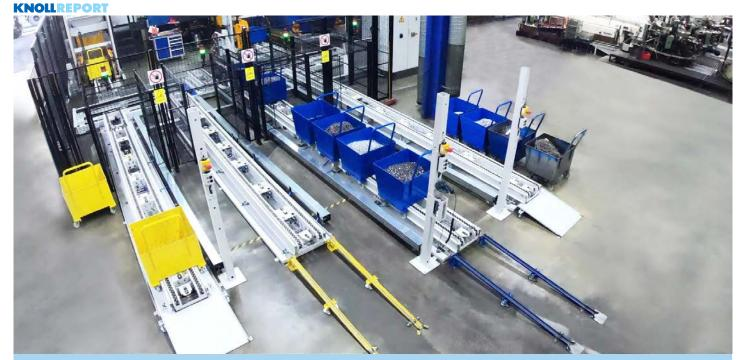
The chip centrifuges are arranged behind the KNOLL transport systems. From there, the degreased chips are taken to the appropriate containers to the right via a portal.
