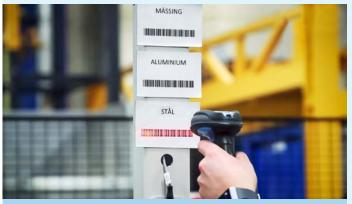
When dropping off the swarf trolley, the employee scans a barcode appropriate for the material.
