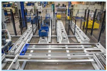
At the end of the buffer lines, the swarf trolleys are transported across a crosswise line to the centrifuges.
