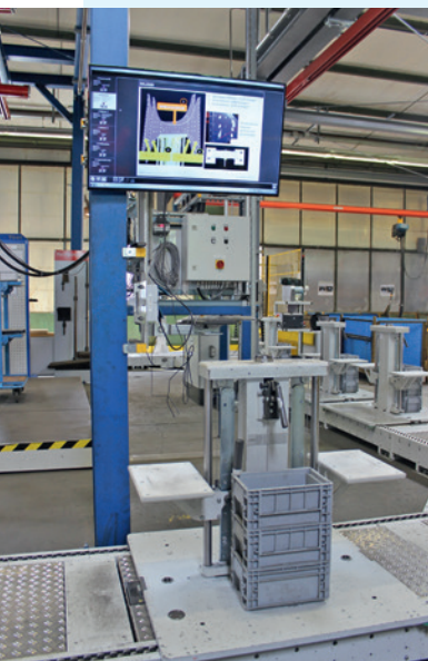
The assembly stand is fitted in the "supermarket." The employee can read from the monitor which components are required.
