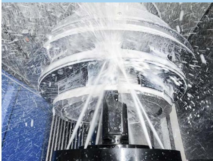
Machining the nickel-based alloy Inconel 718 places high demands on the machine, tool and cooling lubricant.
