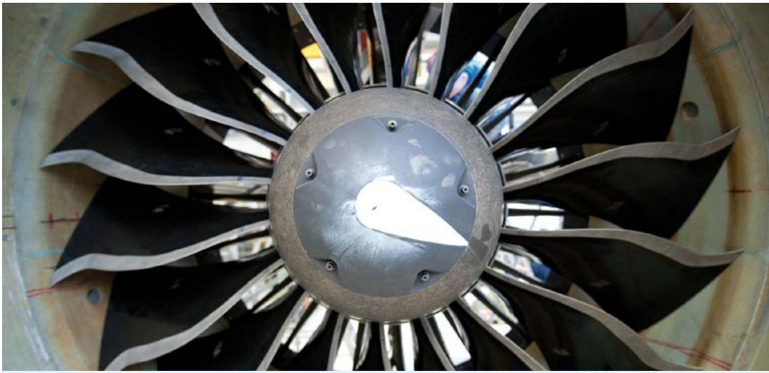
Fan for a Pratt & Whitney GTF™ engine for civil aviation (Airbus A320 neo).
