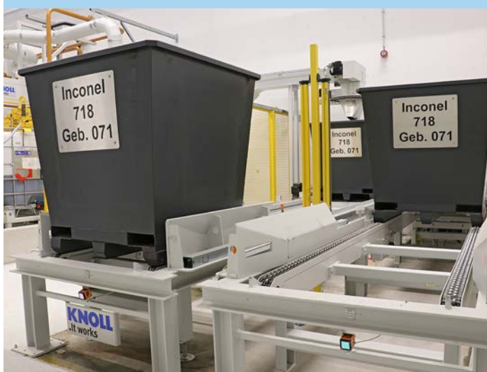
At the end of the sludge remover, the Inconel chips are conveyed via a swivel chute into the special container (in the background). The container station, designed for seven containers, allows unmanned weekend operation.
