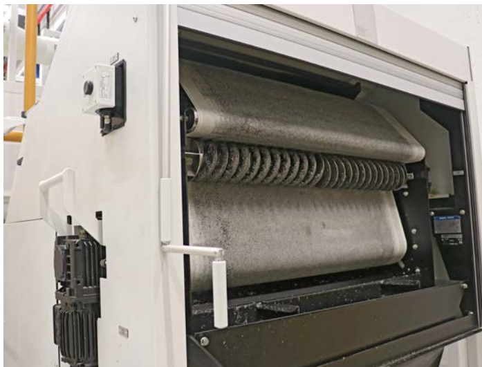
The KNOLL VL1000 vacuum filter cleans the back-flushed medium.
