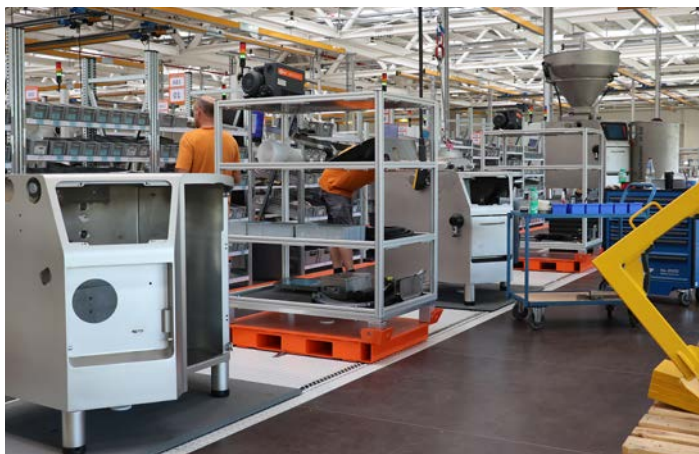
Transport plates with machine frame and trolley assembly are arranged on the conveyor on a rotating basis.
