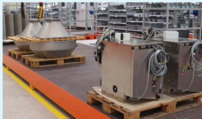
The large parts and pre-assembled components are available on one side of the conveyor belt, on the other side (in the background) are the Kanban shelves with small parts.
