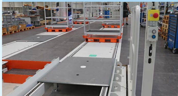
An important element of the conveyor system is the carrier plate, which was designed by KNOLL so that all machine frames can be transported on it.
