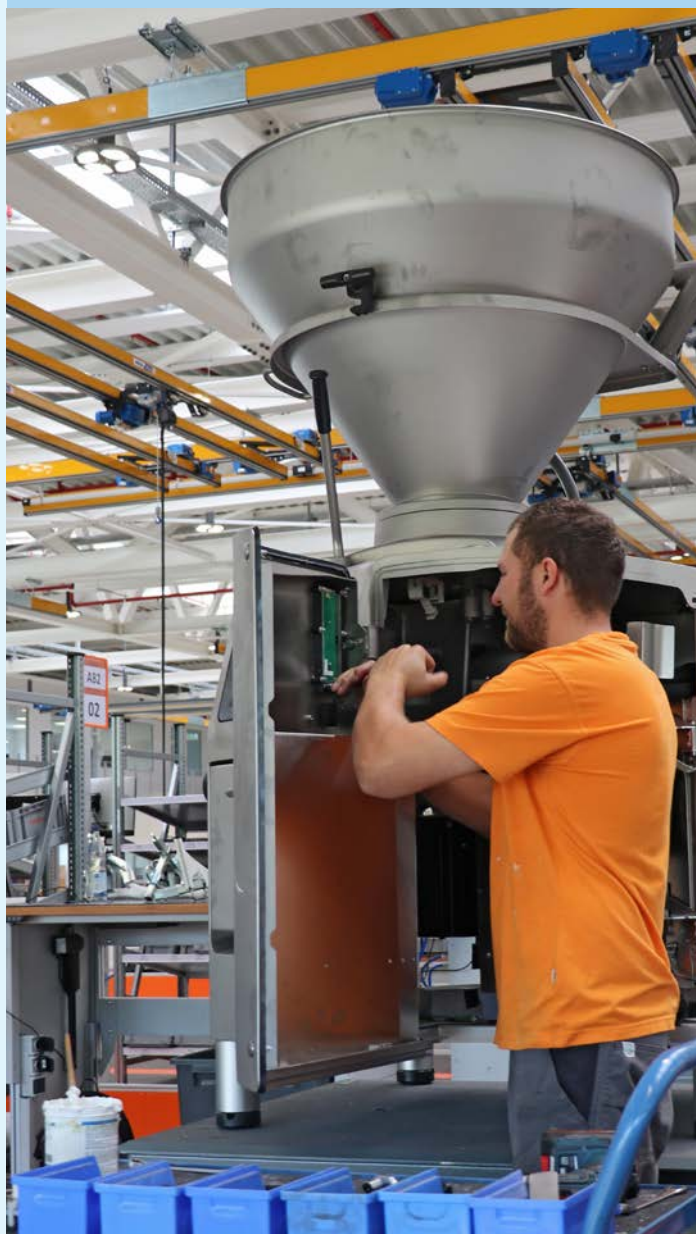
Cycles 1 and 2 are reserved for mechanical assembly, the electrical installation takes place in cycles 3 and 4 (in the picture).
