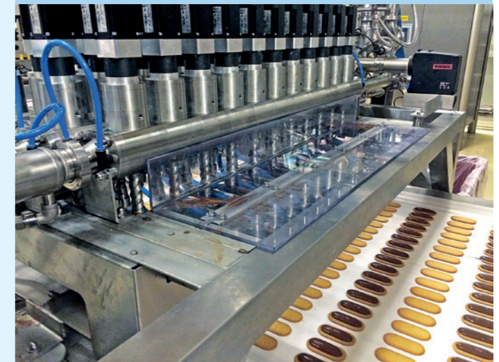
In order to be able to dose crèmes and fillings precisely to the gram, WPI uses KNOLL progressing cavity pumps that are activated with servo gear motors.
