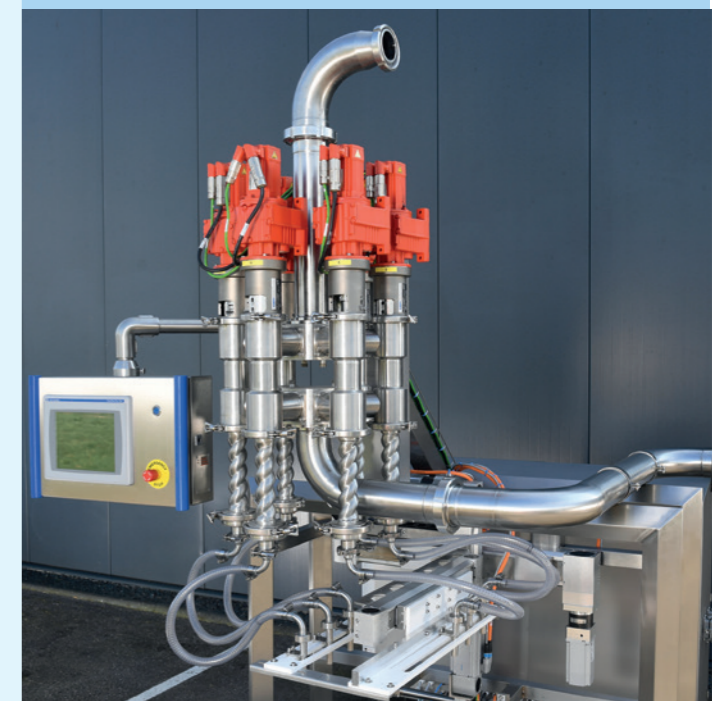
In order to be able to dose crèmes and fillings precisely to the gram, WPI uses KNOLL progressing cavity pumps that are activated with servo gear motors.
