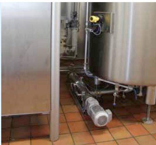
The KNOLL MX30S progressing cavity pump is located between the buffer tank and the tempering unit. It provides a constant delivery rate and thus allows controlled crystallisation of the cocoa butter.
