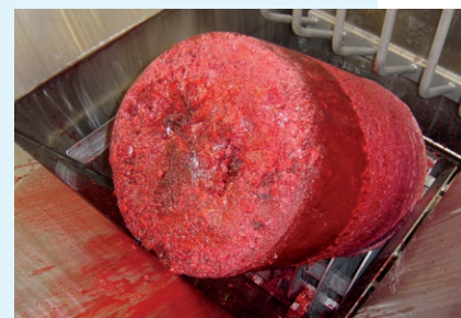
Before processing fruit juice further, the frozen concentrate (here in barrels) is put into the chopper.
