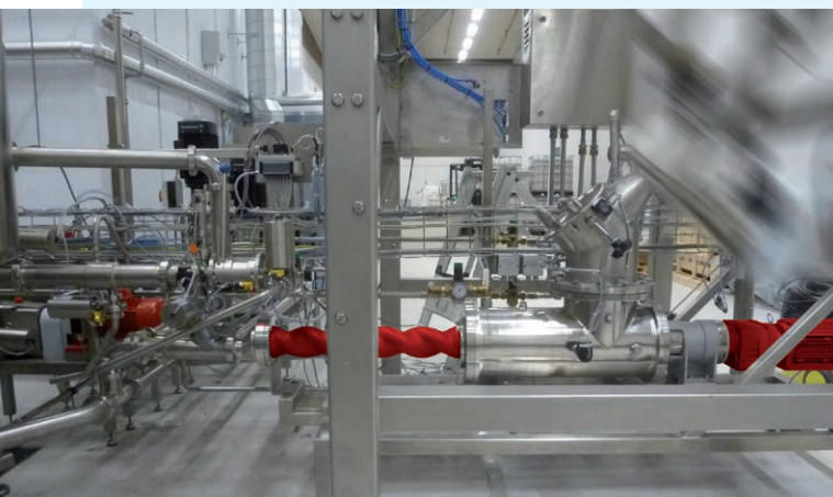
The MX 30R progressing cavity pump was customised for use in the dough mixing process at Isernhäger. Image: Isernhäger
