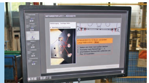
The document displayed on the monitor provides the correct rivet sequence.
