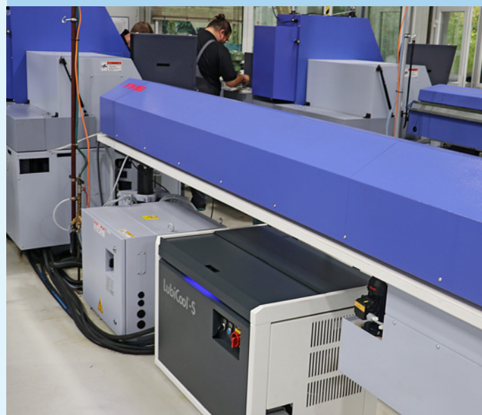
The KNOLL LubiCool®-S high-pressure station is located under the rod loader.
