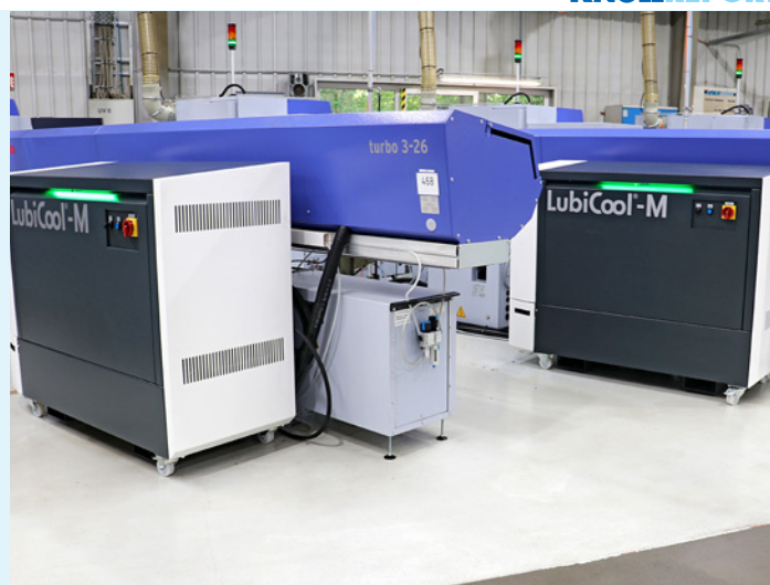
They are the favourites of Feindreh machining specialists: the two KNOLL LubiCool®-M systems, which supply cooling lubricant to the SR-20 long lathes from Star Micronics as needed.
