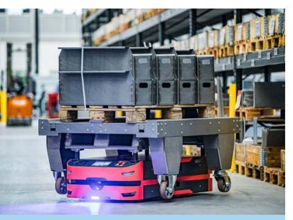
At KNOLL Maschinenbau in Bad Saulgau the majority of the transport orders are now automated. SAFELOG AGVs, which assume the transport of various components from production to warehouse and pick components available in the warehouse and bring them directly to the assembly box or assembly line, are largely responsible for the automated process.
