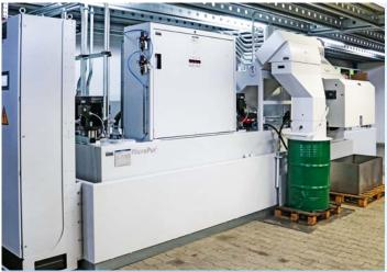
Works perfectly: The KNOLL central system at Schnebelt Präzision consists of a KF-E compact filter (at the back), a MicroPur® ultrafine filter (in the foreground), automatic concentrator (with green drum) and a cooling unit (not in the figure). The compact filter (in the background) ensures dry chip discharge. From the automatic concentrator, the carbide sludge falls into the green drum, largely sorted by type.
