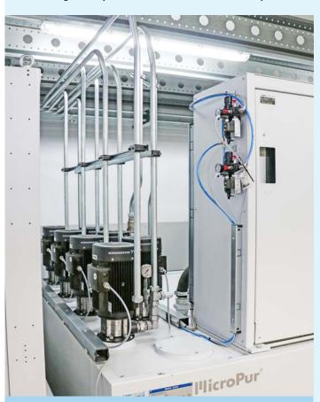
A special request: Unlike the classic central systems, Schnebelt Präzision assigns a clean oil pump with a separate supply line to each grinding machine.
