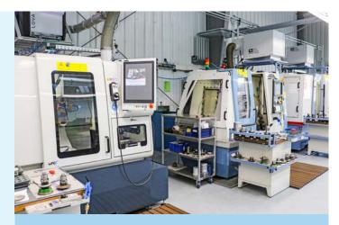
Currently, six 5-axis tool grinding machines are connected to the KNOLL central system.
