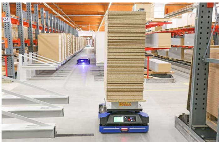
New intralogistics solution at furniture manufacturer Staud: Two KNOLL AGVs, christened Bibi and Tina by the employees, take care of the panel transport from the machine line to buffer stations and on to assembly on the plinth line.
