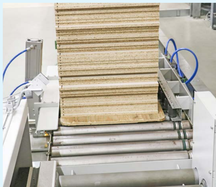
A special device with a stamp ensures that the transport plate is correctly aligned before it enters the transfer station.
