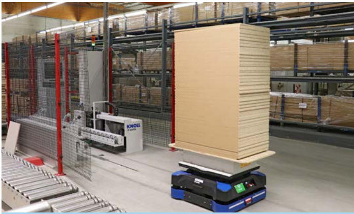
AGV Bibi on its way to the pick-up station on the plinth line.
