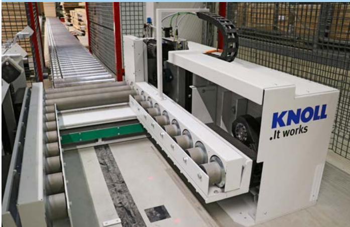
The pick-up station on the plinth line is characterised by solid mechanical engineering. The transport plate is set down on the short roller conveyor. This is followed by a lowering to the low level of Staud's existing transport path.
