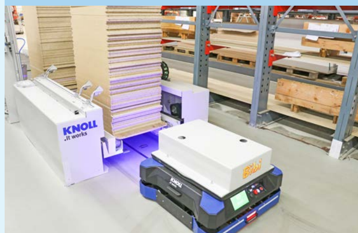
Shortly before the transfer to the AGV: The transport plate is brought to a level at the transfer station by a customer-specific lifting device so that the AGV can drive underneath.
