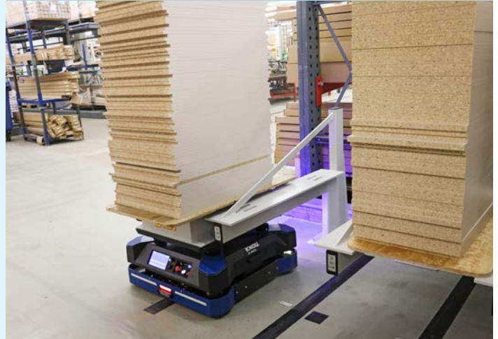
The space is tight. How good that the AGV can turn 360 degrees on the spot and then drive into the buffer station very precisely.
