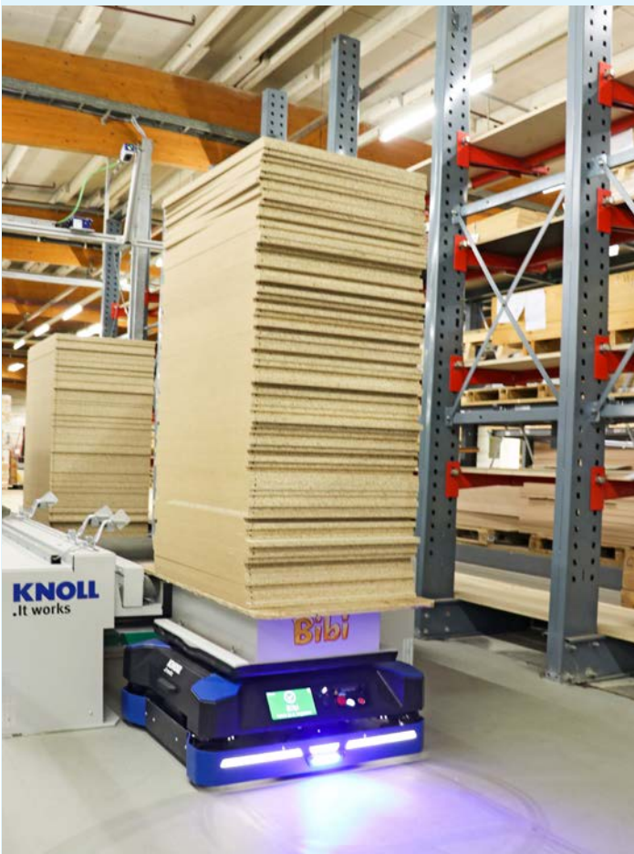
After setting down, the AGV with the panel stack makes its way to a free buffer station.
