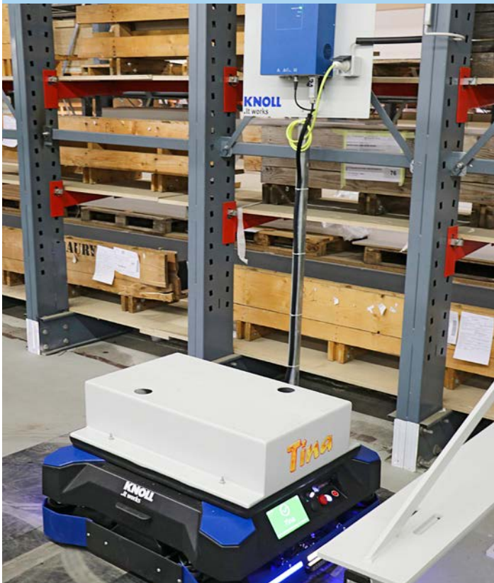
The AGVs spend breaks in transport traffic in the charging station.
