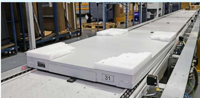
In addition to the conveyor systems and assembly workplaces, KNOLL also designed and supplied the carrier plates, which are compatible with all STIEBEL ELTRON heat pump variants.
