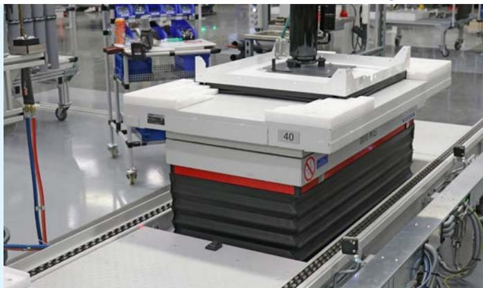
Most of the workplaces are equipped with a lifting table and rotating platform for ergonomic assembly.
