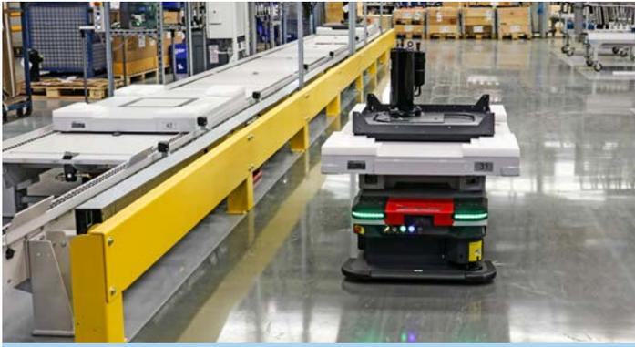
Left in the figure: the first conveyor line. At the two assembly locations, first the base plate and then the compressor for the respective heat pump model are installed.
