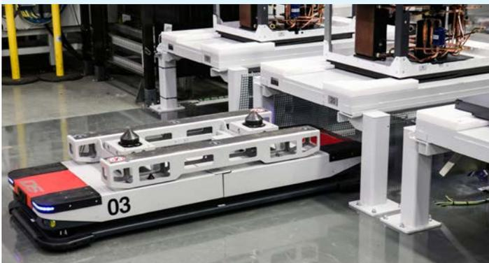
The stationary conveyor technology is networked by means of driverless transport systems. Order management for the transport orders takes place in SAP ME, to which all systems of the entire plant have an interface.
