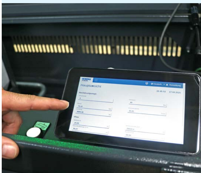
The integrated touchpad enables the monitoring and visualisation of the most important operating data for the system.
