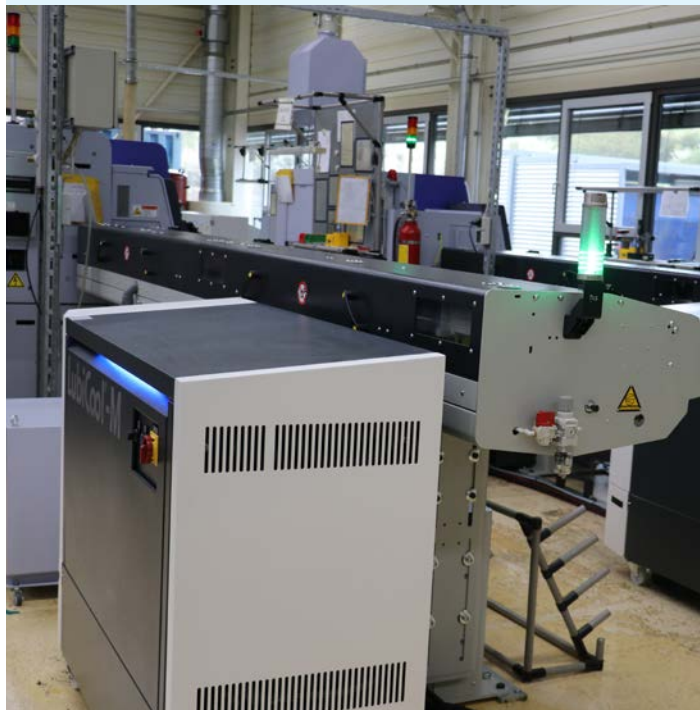
LubiCool®-M units supply the two SP-23 and SV-20R automatic sliding headstock lathes from Star Micronics with cooling lubricant as required.
