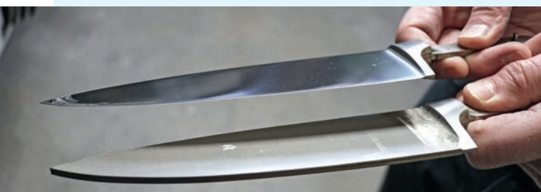
16,000 blades pass through the blade grinding shop every day. There, the laser-cut blanks (top) are ground and polished.
