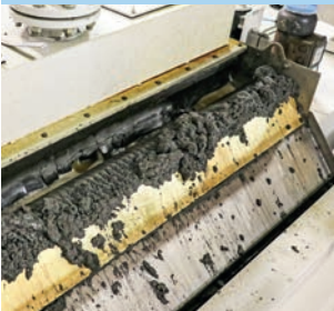
A key to success: the pre-separation via magnetic rollers.
