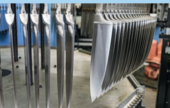
16,000 blades pass through the blade grinding shop every day. There, the laser-cut blanks (top) are ground and polished.
