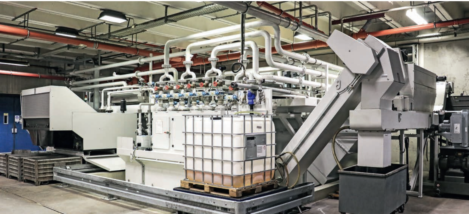
The grinding and polishing processes in ZWILLING's knife production in Solingen are supported by cooling lubricant that is cleaned and tempered in a KNOLL central system featuring multi-stage filtration that requires no filter consumables and is then supplied to the machines. Sedimentation in the type SR sludge remover.
