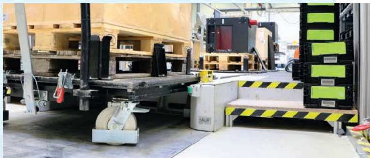
The battery housings to be fitted are on a flat workpiece carrier equipped with a factory-made attachment, which in turn is placed on a transport cart with rollers via tigger train or manipulator.
