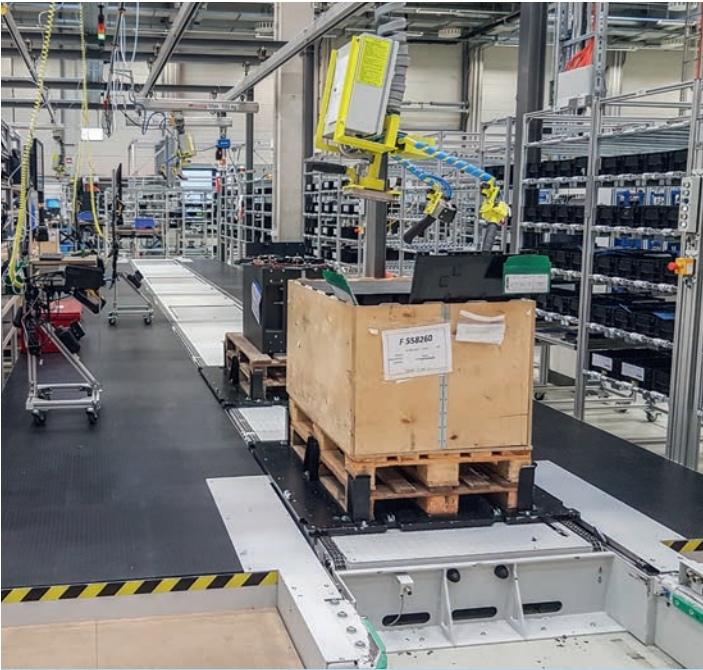
BMZ assembles heavy batteries on KNOLL type TS-S and TS-G transport systems.
