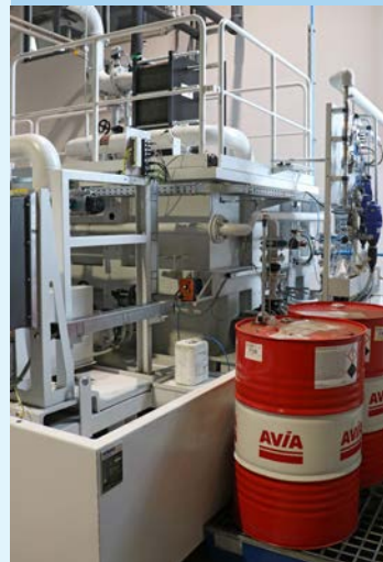
The water-soluble Bantleon cooling lubricant Avilub Metacool ETA which is free of mineral oil is automatically topped up from the red tanks.
