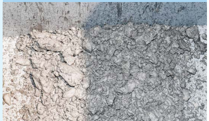
The KNOLL MicroPur® filtration system ensures that even the finest grinding dust is removed from the cooling lubricant and can be disposed of largely dry.
