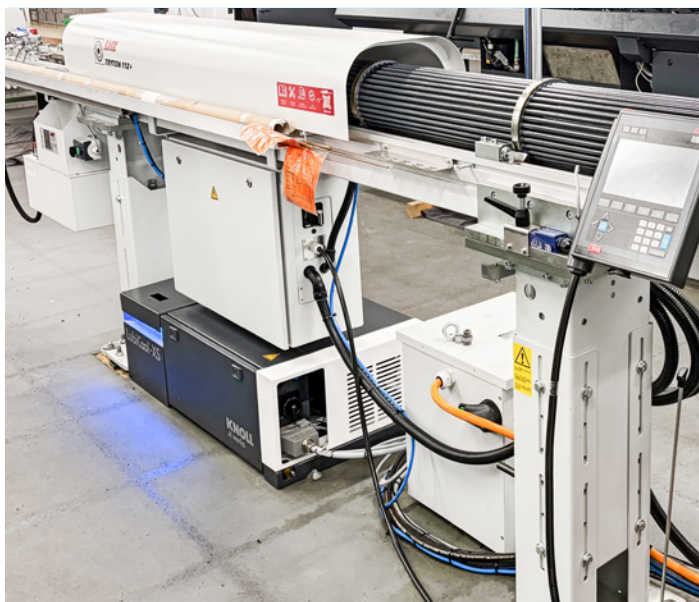
The new KNOLL LubiCool®-XS high-pressure system fits easily under standard bar feeders.
