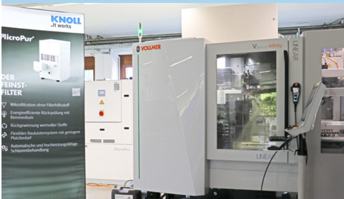
New in the HAM Performance Centre: The machining oil of the tool grinding machine is cleaned by the KNOLL superfine filter MicroPur®.
